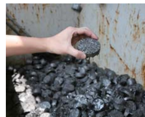
▲ Solidified sludge at the KOFU Plant
